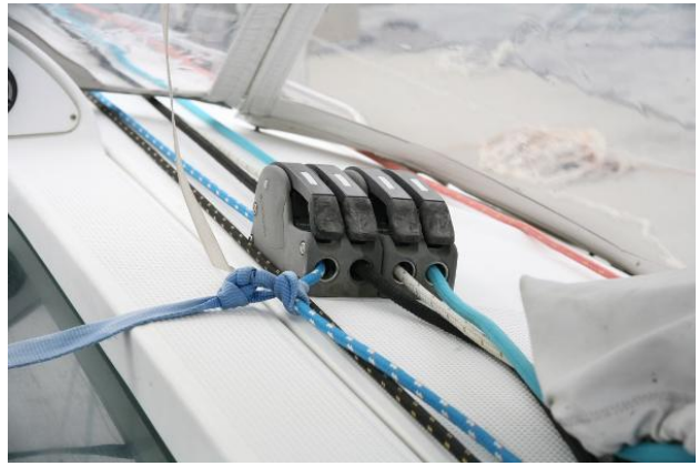
36' Beneteau 36.7 Southern Cross line clutches
